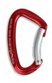
Type: В 96 mm Length: 59 mm Width: Weight: 44 g Major axis: 24 kN 8 kN Minor axis: 7 kN Open: Material: Light alloy CE - EN 12275 - UIAA Norm:
