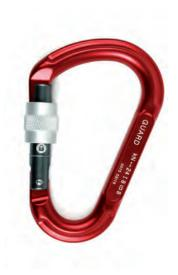
H/B Type: Length: 120 mm Width: 76 mm Opening: 22 mm Weight: 86 g Major axis 24 kN Minor axis 8 kN Open 8 kN Material: Light alloy
