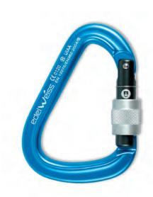
Type: H/B Length: 105 mm Width: 66 mm 20 mm Opening: Weight: 66 g 28 kN Major axis: Minor axis: 8 kN 8 kN Open: Material: Light alloy
