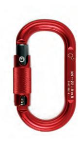
Type: X/B Length: 110 mm Width: 61 mm Opening: 16mm Weight: 81 g Major axis: 22 kN Minor axis: 8 kN Open: 8 kN
