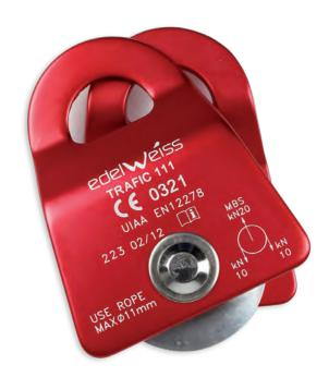
Height: 72mm Width: 58mm Sheave: 27,5mm 1 rope max.: 11mm Weight: 120 g
