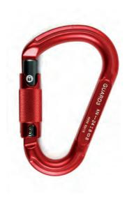
H/B Type: Length: 120 mm Width: 76 mm Opening: 22 mm Weight: 100 g Major axis: 24 kN Minor axis: 8 kN Open: 8 kN Material: Light alloy
