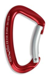
Type: В 96 mm Length: 59 mm Width: Weight: 44 g Major axis: 24 kN 8 kN Minor axis: 7 kN Open: Material: Light alloy CE - EN 12275 - UIAA
