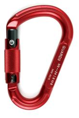
H/B Type: Length: 120 mm Width: 76 mm Opening: 22 mm Weight: 86 g Major axis 24 kN Minor axis 8 kN 8 kN Open Material: Light alloy
