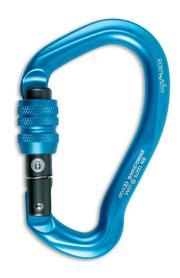
Type: H/B Length: 105 mm Width: 66 mm Opening: 20 mm Weight: 66 g Major axis: 28 kN Minor axis: 8 kN 8 kN Open: Material: Light alloy
