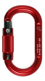
Type: X/B Length: 110 mm Width: 61 mm Opening: 16mm Weight: 81 g Major axis: 22 kN Minor axis: 8 kN Open: 8 kN Material: Light alloy
