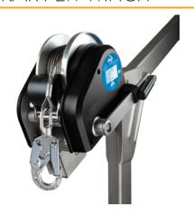
Hand crank winch for easy and jerk-free lifting and lowering of persons and loads according to Directive 2006/42/EG with 30 m stainless steel rope of Ø 6mm (min. breaking load 18.76 kN). SWL is 300 Kg.
