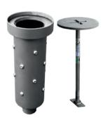
Flush floor sleeve with 3/8" drainage pipe connection to be installed to existing concrete by core-drilling and resin fix.
