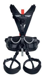
You want freedom of movement when working on the roof, and the ROOF MASTER harness with its many features and unique Singing Rock MOTION SYSTEM guarantees it. Its movable attachment point is openable, which makes it easy to connect a chest ascender or detach the shoulder straps. So, you can choose between a full-body and a sit harness, it's up to you.
